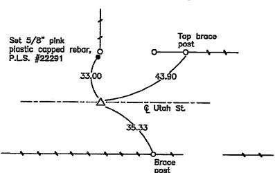
NOTE: ALL TIES ARE PLUMB MEASUREMENTS TO ORANGE SURVEY MARKER UNLESS NOTED.
