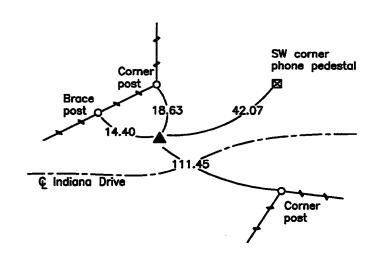
NOTE: ALL TIES ARE PLUMB MEASUREMENTS TO ORANGE SURVEY MARKER UNLESS NOTED.
