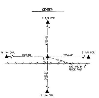
JAN. 26, 2022-PLS 14416: SET 5/8" X 30" REBAR WITH YPC #14416 AT INTERSECTION OF LINES BETWEEN OPPOSING 1/4 CORNERS. LOCATION IS SUPPORTED BY FENCE LINE AND FIELD LINE EVIDENCE NORTH, SOUTH, EAST, AND WEST.
